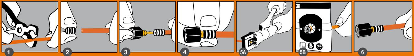
Cut the QUADRA capillary hose to the required length using the special WXA004 cutter.
