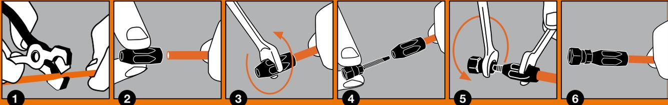
1 Cut QUADRA DN4 capillary hose to the required length using our cutter for capillary hoses type WXA004.
